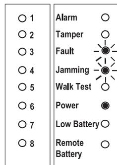
Radio frequency blocked. Call Scantronic technical support.
