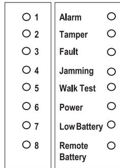
If the battery voltage is low then the power LED goes dark and the panel beeps every 30s. When the battery voltage falls below 8V (approx) then the panel stops operating.
