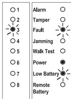
Low battery on zone detector. Replace battery.
