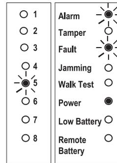
Zone activated during exit time or during re-arm period after an alarm. Enter user code twice.
