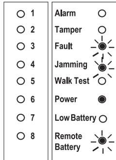
Remote setting transmitter jammed on. Check for obvious causes, e.g. test switch turned on.
