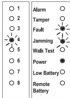
Jamming present on zone 4. Check for interfering radio signals. Activate detector/transmitter and enter user code twice. If fault persists then call Scantronic product support.
