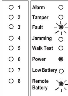
Low battery on remote setting transmitter. Replace battery.
