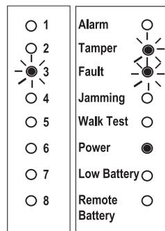
Tamper on zone active during exit time or during re-arm period after an alarm. Enter user code twice.
